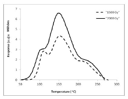
Figure. 2 Glow curve of topaz: glass composite in ratio 2:1, sintered at 1000 °C for one hour, irradiated for 1500 and 2000 Gy doses with Beta irradiator and TL read out with Harshaw (TLD-3500) at the heating rate of 5 °C/s.
