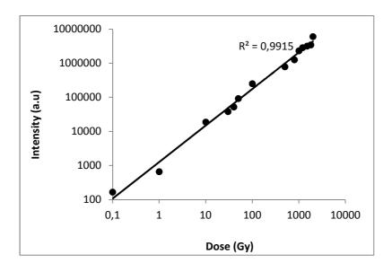
Figure. 4. Intensity of Peak 2 of topaz composites irradiated for the various doses with Beta irradiator and TL read out with Harshaw (TLD-3500) at the heating rate 5 °C/s.
