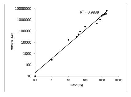
Figure. 3. Intensity of Peak 1 of topaz composites irradiated for the various doses with Beta irradiator and TL read out with Harshaw (TLD-3500) at the heating rate 5 °C/s.
