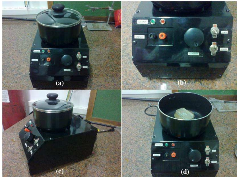
Figure 3: Spinner in its final configuration: (a) front view, (b) control panel, (c) lateral view, (d) sample holder.
