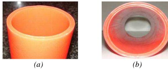
Figure 4: Sample achieved using two PVC pipes and vaseline liquid demoulding agent applied to the inner and outer walls of the inner tube and the inner wall of the outer tube.
