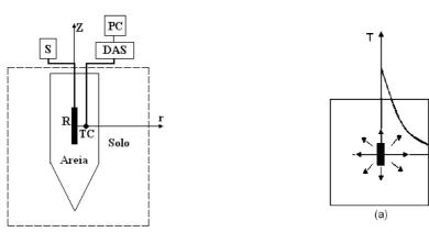
Figure 1 – Outline of the transducer: S = Electricsource, TC = thermo-couple, R = Electric resistance, DAS = Data Acquisition System (analogic/digital plates), PC = Personal Computers
